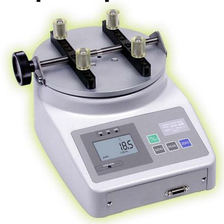
The new, easy-to-use Check•Line® DTX2 Cap Torque Tester accurately measures twist on and twist off force. The tester offers programmable high/low setpoints for go/no-go testing. ORANGE lights up for measurements less than Low setpoint, GREEN for between High and Low setpoint, and RED for over High setpoint.
